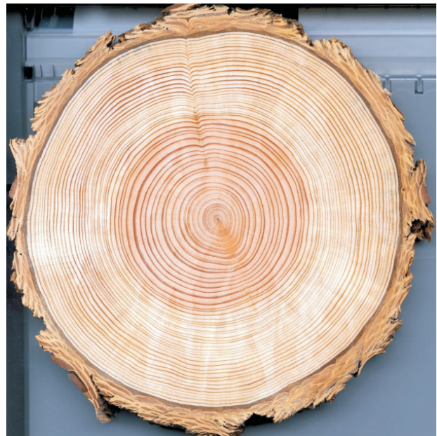
FIGURE 5. By counting growth rings, the age of this Douglas-fir at the time it was felled is determined to be 50. (Courtesy, Henri Grissino-Mayer)
